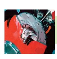
Turbo compressors are the type of compressors that provide kinetic energy to the air or gases by the centrifugal force generated by the impellers and convert this kinetic energy into pressure energy in the diffuser by reducing the air flow path.
