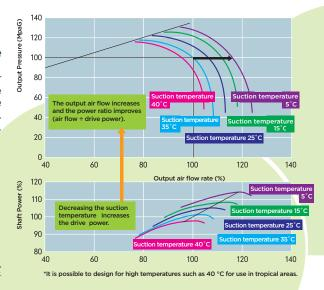
\*If the output flow rate exceeds the maximum capacity, motor overload protection function shall prevent intake of air.
